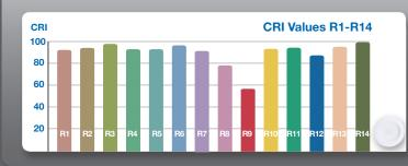
The CRI<sup>SP</sup> SERIES DOWNLIGHT 18W lamp features a typical CRI 90, R9 55 and R13 94, providing crisp and vibrant colors across the whole spectrum. Its exceptional R9-R14 values (R9 & R13) provide redder reds, natural looking skin tones and whiter whites. In addition, this lamp's color temperatures fall within a 4-step Macadam ellipse to ensure minimal color deviation across lamps.
