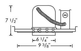
"Designed for use with trims that have integral socket brackets and designed to be contractor friendly for *quick installation*."
