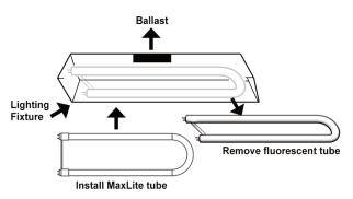
Figure 2. - Install MaxLite Retrofit U-Bend lamp
