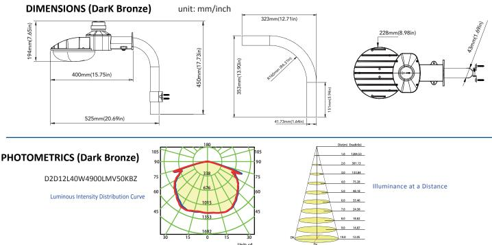
Beam Angle(B): H146.9 V146.5 Field Angle(F): H160.0 V159.6
