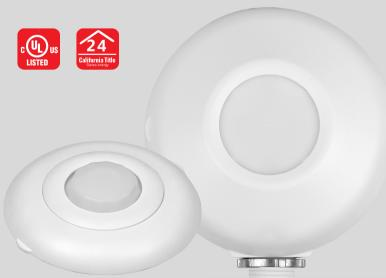
The MPC-50HD is a commercial grade line voltage high bay ceiling sensor that operates dimmable lights using passive infrared (PIR) technology. This unit is specifically designed for high bay and fixture mounted applications and it features interchangeable 360° fresnel lenses that provide up to 1200-2800 sq.ft of coverage area for ceiling heights from 8-50ft.
