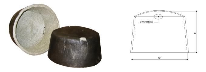
The FF109-300 Fire Rated Cover is designed to reduce the ability of the insulation catching fire. Makes your recessed lights fire rated and gives you piece of mind that you are protected against accidental insulation fires. The FF109-300 is easy to install and fits most IC Rated fixtures. In a fire, the intumescent material expands 5 times of its original thickness, closing the vent holes and preventing flames to spread.
