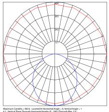
Maximum Candela = 483.6 Located At Horizontal Angle = 0, Vertical Angle # 1 - Vertical Plane Through Horizontal Angles (0 - 180) (Through Max. Cd.) # 2 - Horizontal Cone Through Vertical Angle (1) (Through Max. Cd.)
