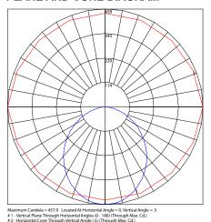
Photometric values based upon tests performed in compliance with LM-79. IES files can be downloaded at www.ilp-inc.com
