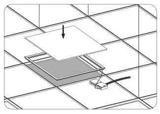
Fix the LED Frame light into lightgage steel joist, cover the ceiling plaster slab.
