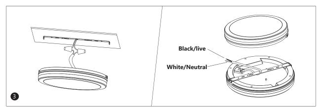
3. Connect black wire to live wire, white wire to neutral wire, and secure using wire nuts.
