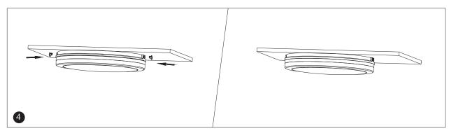
4. Fixing the lamp body on bracket and fix tightly
