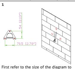
First refer to the size of the diagram to drill holes in the wall.
