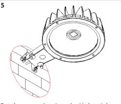
Put the cover plate into the U-slot, tighten the screws.
