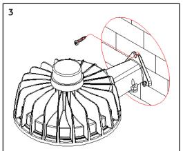
Hook the lamp by two screws. Attach the top screw. Finally tighten all screws.
