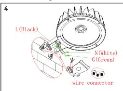
Pass the wire through the hole of the cover plate. Connect the wire to the same color (correspond to wire N, L and G) together with a wire connector.
