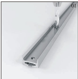
Drill holes for power cord and to mount to surface.
