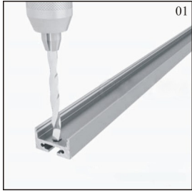
Drill hole for power cord.
