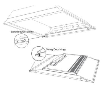
3.1 Locate the swing door supports located on each end of the Lamp Bracket. Install the swing door hinges into the keyholes on the Lamp Brackets.
