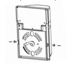
4.Install the fixture body to quick installation plate and tight the screws.
