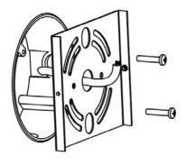
2.Fix the quick installation plate to wall.
