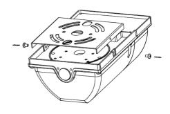
1. Loose screws to take the quick installation plate apart.
