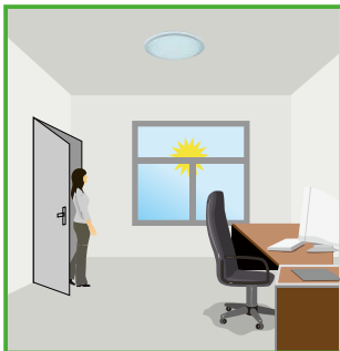
With sufficient natural light, the light does not switch on when presence detected.
