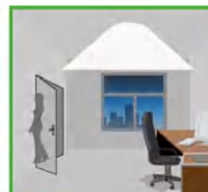
The light dims to stand-by period after hold-time and stays on selected minimum dimming level
