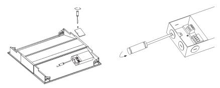
**3.)** Through the conduit, the power feed is connected to the wiring terminal; make sure the connection is solid and reliable.
