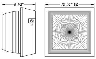
THREE 0.50" CONDUIT ENTRY POINTS ON SIDES ONE 0.50" CONDUIT ENTRY POINT ON BACK
