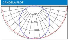
Maximum Candela = 1775.4 Located At Horizontal Angle = 292.5, Vertical Angle = 4
