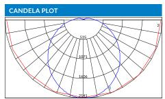
Maximum Candela = 2141.1 Located At Horizontal Angle = 292.5, Vertical Angle = 4 # 1 - Vertical Plane Through Horizontal Angles (292.5 - 112.5) (Through Max. Cd.) # 2 - Horizontal Cone Through Vertical Angle (4) (Through Max. Cd.)
