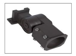
Slipfitter Mount An optional cast aluminum mast arm adapter secures fixture head to nominal 2"(2-3/8"0.D. pipe size) horizontal steel tenon arm.
