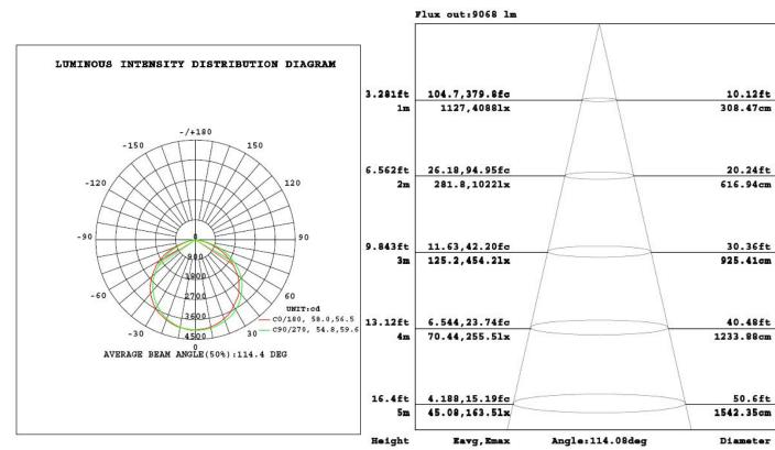
Note: The Curves indicate the illuminated area and the average illumination when the luminaire is at different distance.
