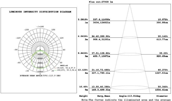
illumination when the luminaire is at different distance.
