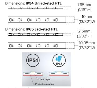
When using standard snap connectors, it is recommended to scrape off the coating from each conductor to ensure a proper connection. When using heavy duty snap connectors, this is only necessary for IP65 and IP68 types.
